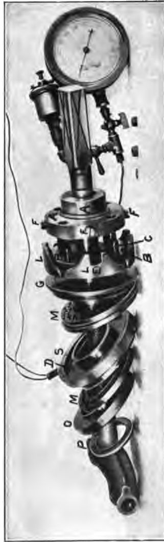
Fig. 95.—Transmission Dynamometer Taken Apart to Show Construction.
